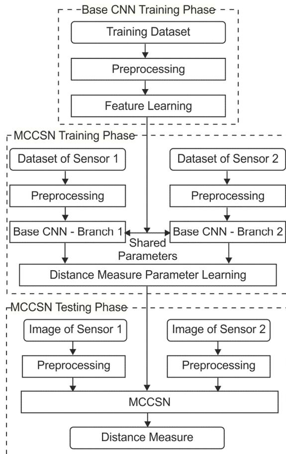
Fig. 4. The framework of proposed system.
